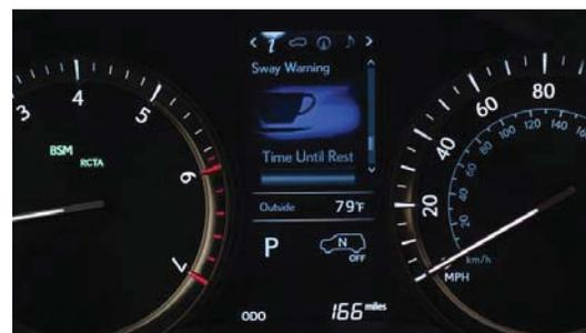
The Vehicle Sway Warning function can be activated or deactivated, and its sensitivity can be changed, on the Multi-information Display customization display using the DISP switch on the steering wheel.
