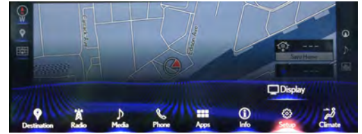
STEP 2 Slide your finger across the touchpad to highlight Setup . Push down, or double tap on the touchpad to select.
