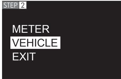
**STEP 2** Press the **DISP** switch again to highlight "VEHICLE" from the list. Press and hold the **DISP** switch to view the customization options. Press to scroll, or press and hold to select highlighted option.
