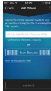
To add a vehicle, enter the VIN manually or scan the VIN Barcode from vehicle, and click validate.
